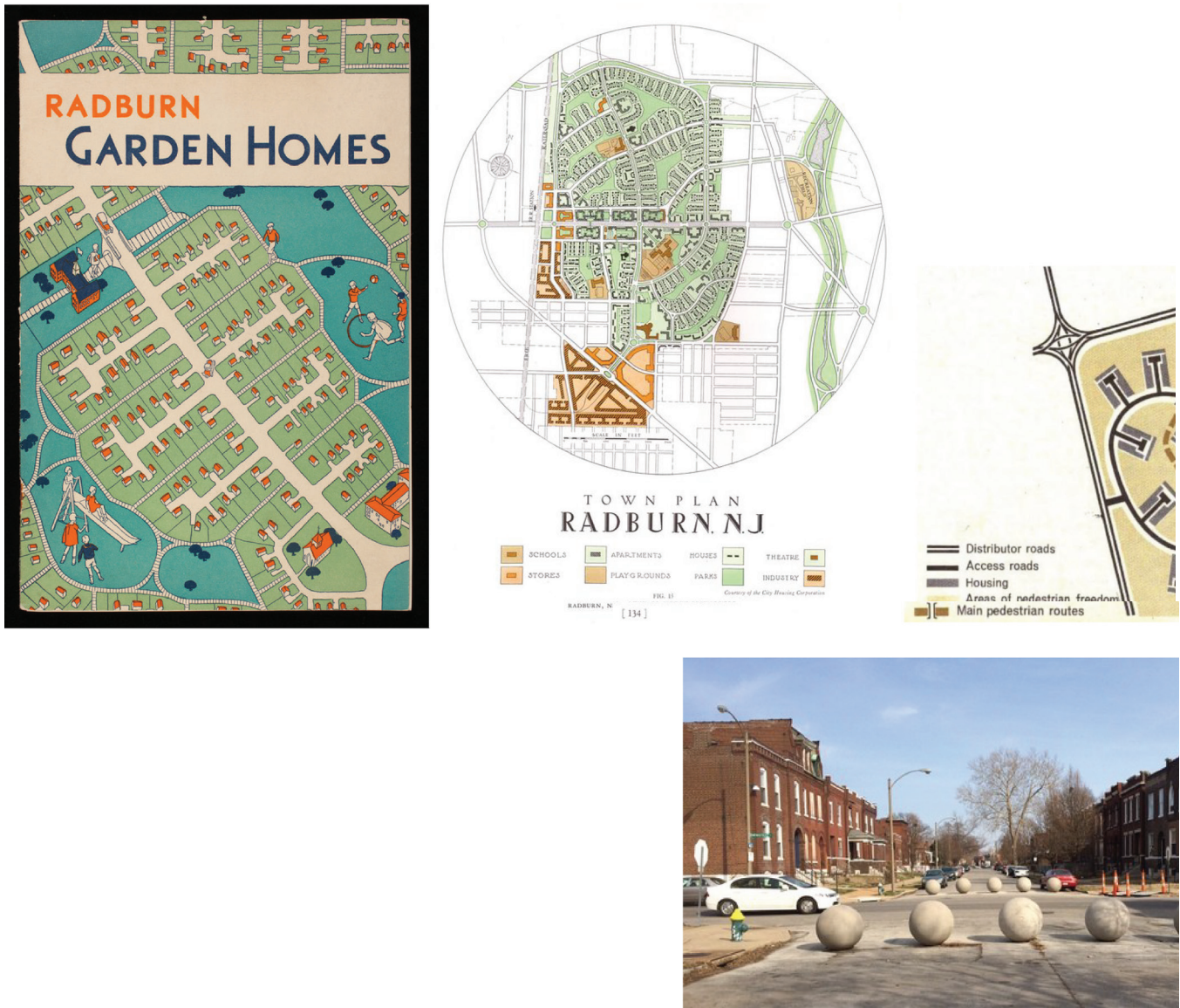
Figure 2. Top: The town of Radburn, which is frequently cited as an early contemporary example, is where the layout became basis for modern planning. [Left] Original garden homes included cul-de-sacs with adjacent walkable green spaces. Image Credit: City Housing Corporation. Source: Historic New England. 3 [Middle] The Radburn Superblock. Drawing Credit: Clarence Stein, Henry Wright, and Marjorie Cautley. [Right] Plan interpretation of the Radburn model. Drawing Credit: Colin Buchanan (1963, 69). Bottom: Concocted sacked conditions facing each other and blocking the streets grid in St. Louis, MO. Image Credit: Lindsay Toler. Source: www.riverfronttimes.com . 4
